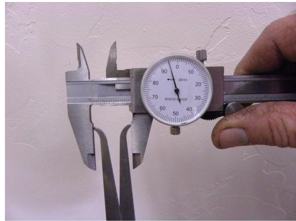
Measure the diameter of the trucks using the outside caliper. Record the data on the Worksheet grid, and enter the average on Line 4. Divide by 2 to get the Radius on Line 5.
