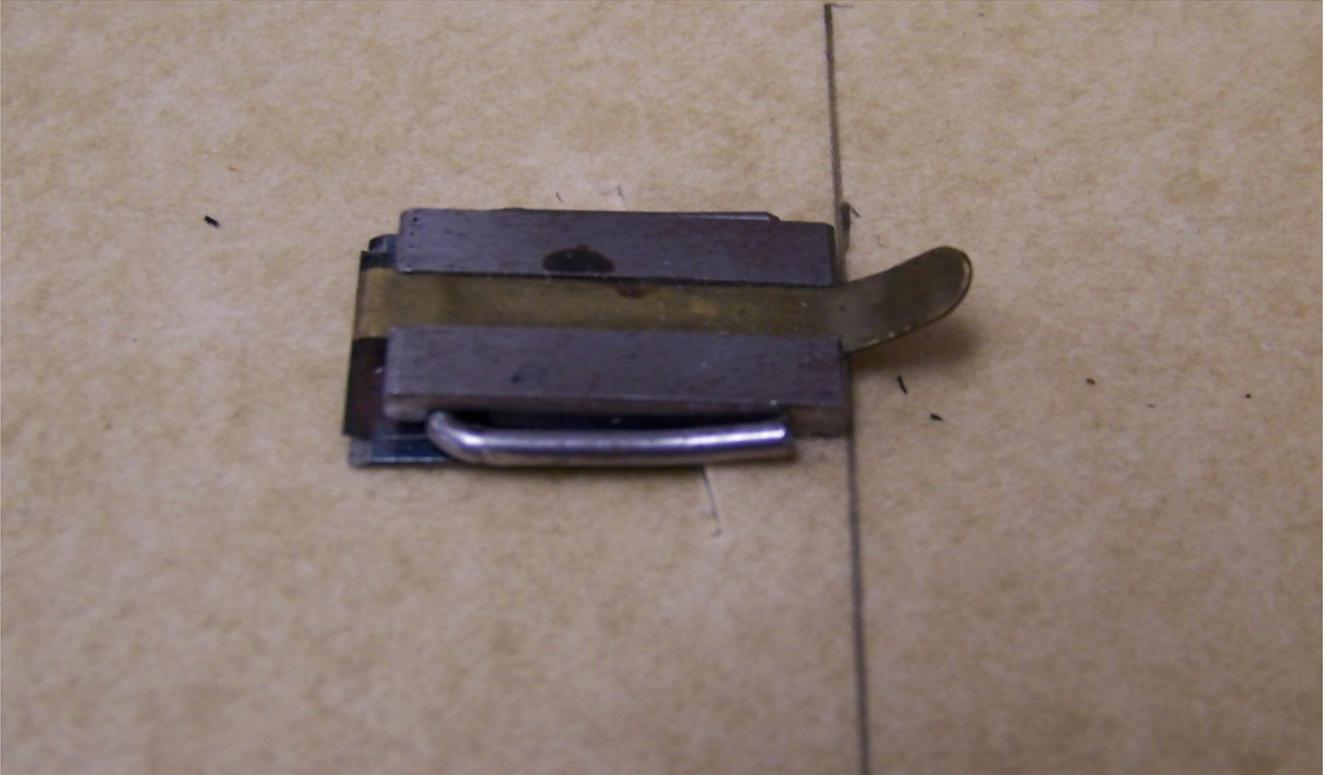
10. Remove the gauge pins from the top sheet after every run, unless you're certain there will be no change in the lockup (and that *you* will be the next one to use the press). The next form locked up and put in the press may be aligned to smash the pins.
