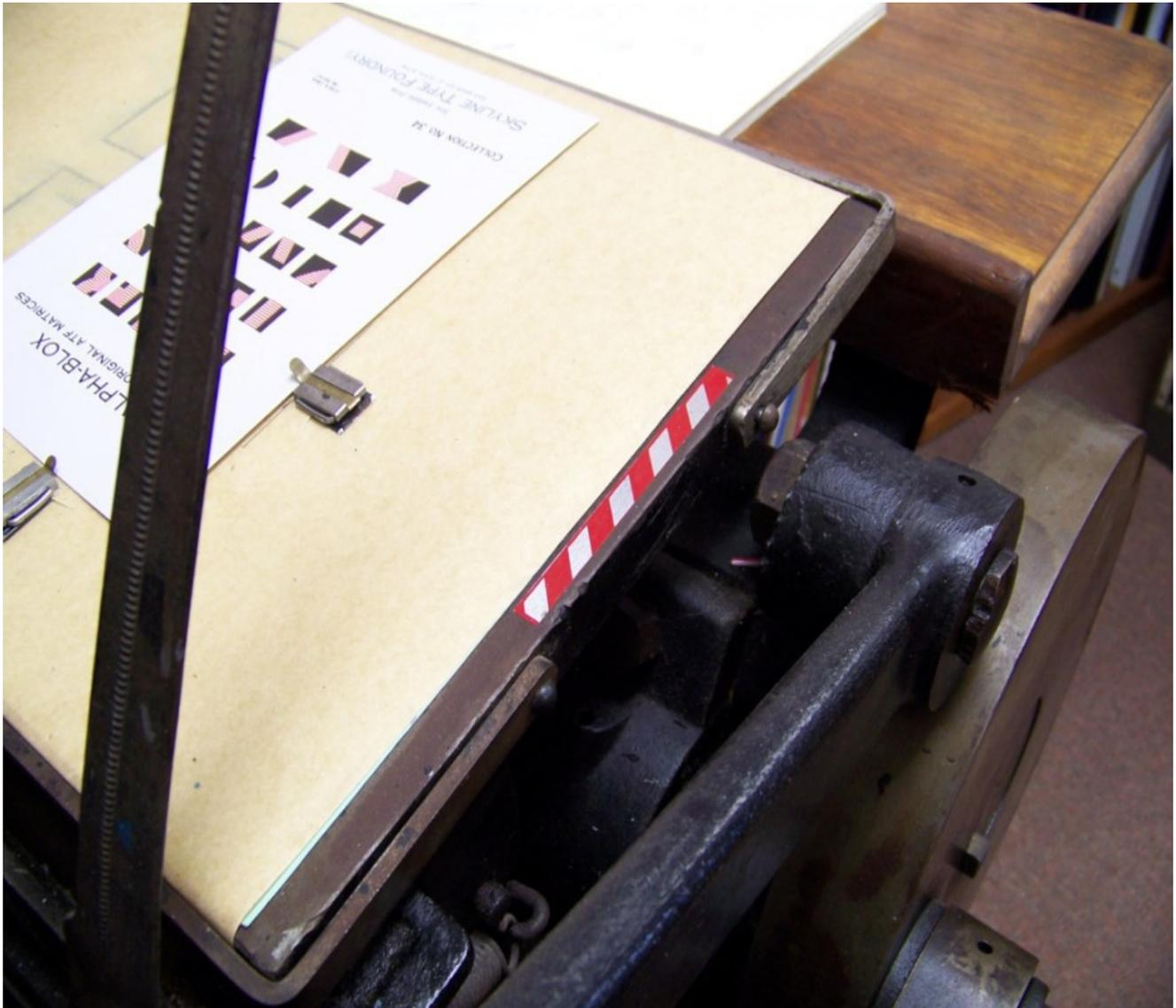
2. If your form includes any Linotype or Ludlow slugs, rout the shoulders of them down on a saw. (Yeah, I know, who uses a linecaster these days?) The ends of untrimmed slugs are all too effective at smashing gauge pins.
